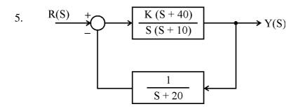
In the above figure, find the gain K that results in marginal stability. Determine the oscillation frequency.
